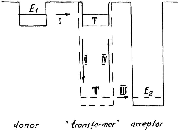
Fig. 2. 'Four-step' performance regime of carrier-transformer  $T$  [3].  $T^0$ ,  $T^-$  states describe the 'initial', and  $T^+$ ,  $T^-$  – the 'final' conformations ( $T^0$  and  $T^-$  are metastable). Electron transitions I, III may be of a tunnel-like nature.
